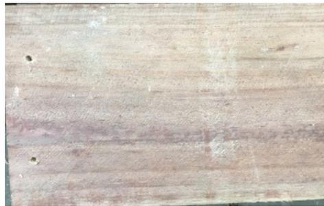
2. On the 4 supports/caps, drill 4 holes (all the way through). The holes should be located 100mm in from the ends and 25mm in from the sides. Refer photo below.
